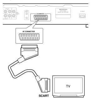
This connector can output composite video, S-Video, or RGB video. The default setting is composite, which should work with all TVs. Consult the manual that came with your TV to see if you can use one of the higher quality settings. See page 41 for how to change the video output.
